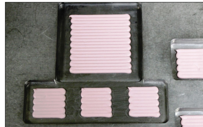
Figure 4: Multiple location casting
