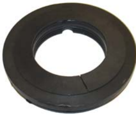
Failed Seal Resulting from Improper Fit
