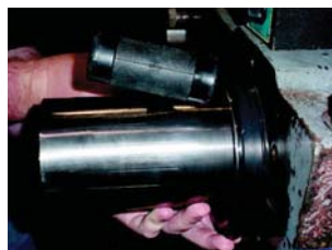
Installing the Seal
