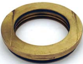
Failed Seal Resulting from Improper Installation
