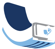
10 The OD can be ground, OD sealant applied and the edge of the case can be rolled as needed
